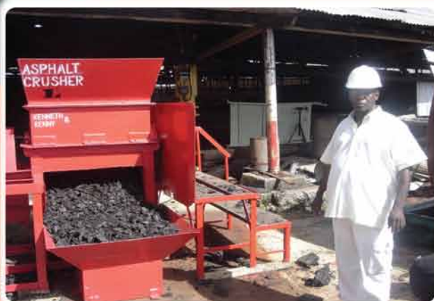
Mr. Kenneth Roberts Assistant Engineering Superintendent with his locally engineered crude asphalt crusher.
